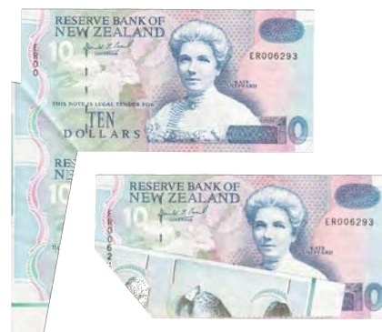
This error was caused by a fold in the paper, after the banknote sheets were printed but before the serial numbers were printed and the sheets guillotined. This creates a "flap."
