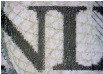
Above: Inkjet printing. Note the stair steps on the diagonals and curves. Digital processes do not always handle angles well. Note also the left arm of the Y extending into the L's space at right.
